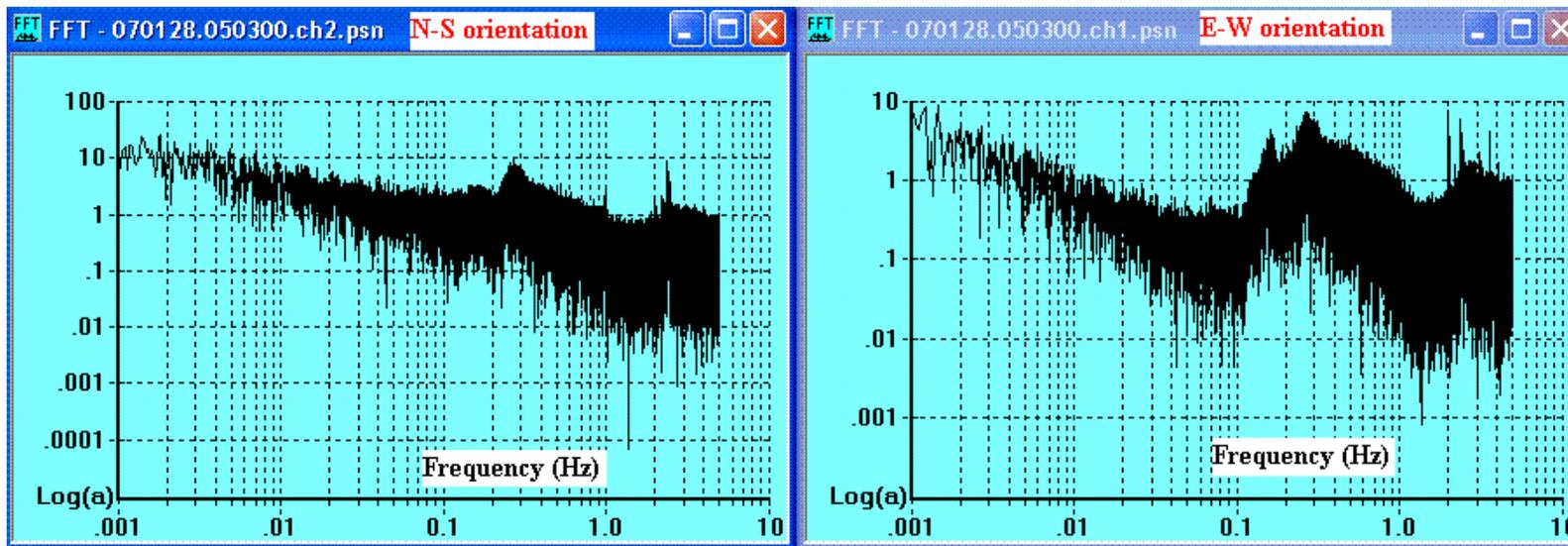
**Figure 1.** Illustration of the difference in response to secondary microseisms between the North-South pendulum and the East-West pendulum for a VolkMeter located in Macon, Georgia.
