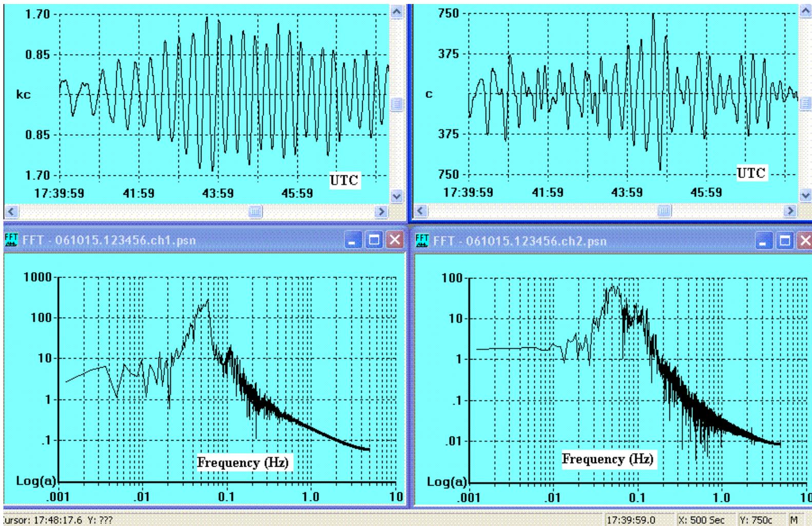
**Figure 4.** Time-domain (500 s duration) and associated frequency-domain portions of records following the Mag. 8.1 earthquake of 13 January 07 east of the Kuril Islands. Low-pass filtering was done at 0.1 Hz.
