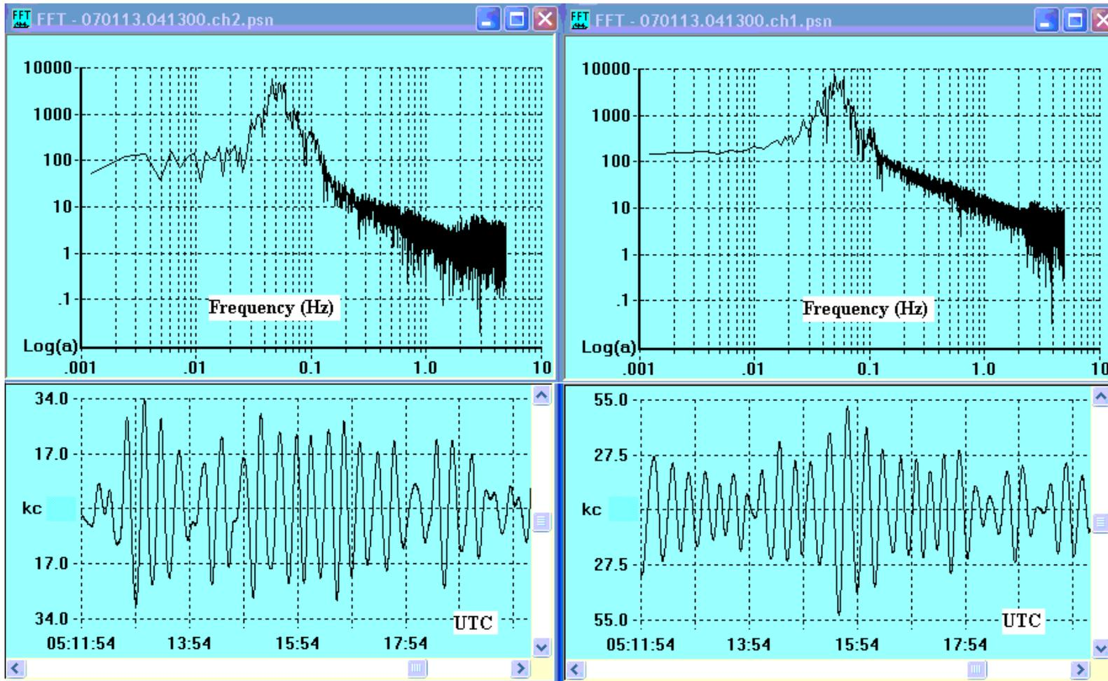
**Figure 3.** Time-domain (500 s duration) and associated frequency-domain portions of records following the Mag. 6.7 earthquake of 15 October 06 off the Kona Coast of Hawaii. Low-pass filtering was done at 0.1 Hz.
